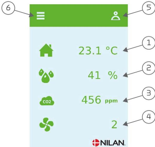
1. Shows the current room temperature in the house, measured via the extract air.
